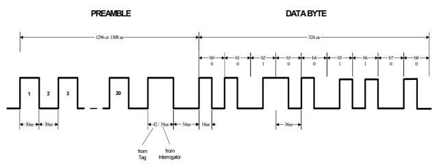
Pulse width in microseconds. Data byte transmitted significant bit first. Byte shown is code 0x64.
